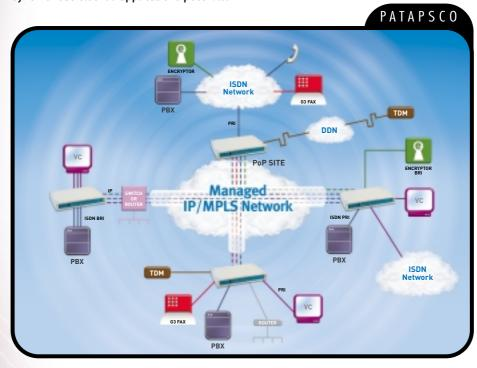
The diagram illustrates a few possible ISDN switched and nonswitched TDM applications with break out from a PoP site.
